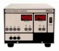
The VFC 501 Series is a variable AC power source designed to deliver power at a selectable frequency between 47Hz to 424Hz. The unit uses PWM technology and generates a pure sine-wave output with typical distortion of less than 5%. The output voltage is continuously adjustable from 0 to full scale.
